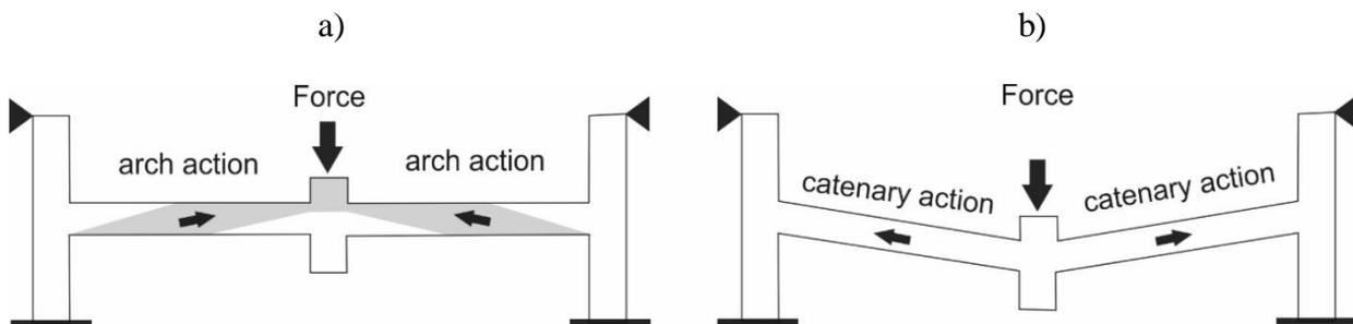
*Figure 11 - Mechanisms of resistance to the disproportionate failure of floor structures and roofs: arch / shell (a); catenary / membrane (b)*
