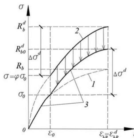
Figure 3 - Schematic diagram of the deformation of reinforced concrete under static-dynamic loading mode caused by a special emergency action [74]: 1 - single short-term (quasi-static) loading; 2 - single dynamic (impulse) loading; 3 - static-dynamic loading
