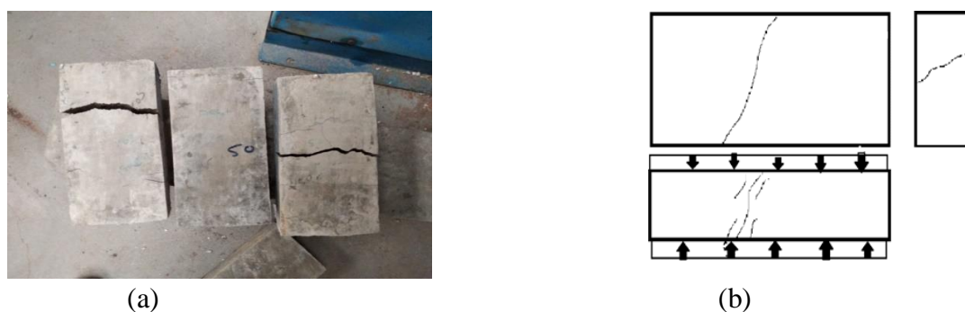
Figure 11 - Failed Brick Samples (a), Failure Pattern of Brick (b)
